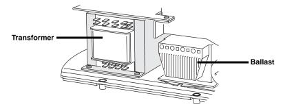
3. On the transformer, move the brown and blue wires (those with insulated spade plugs) to the transformer taps shown for your mains voltage (see Table 2).
